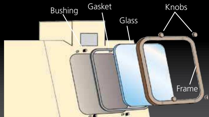
**Safety-Glass Window** (14" x 22") provides large viewing area, can be changed in a few minutes without tools and has rounded corners for safe handling.
